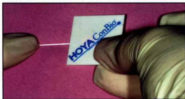
Fig. 2 Before each patient use, 2-3mm on end of optical fiber nicked with small cleaving stone and cut off cleanly.
