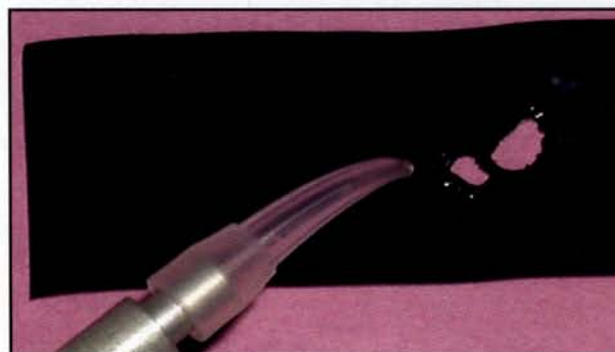
Fig. 4 Optical fiber activated by tapping it lightly on dark surface. Small holes on carbon articulating paper indicate laser is ready for use.
